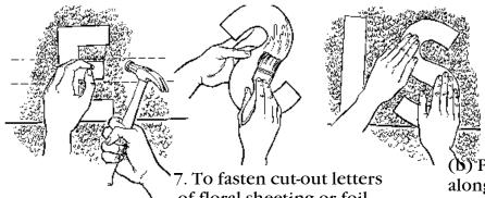
6. To fasten cut-out wallboard letters, place bottom of letter along guide line string and nail to center board of apron 7. To fasten cut-out letters of floral sheeting or foil paper:
